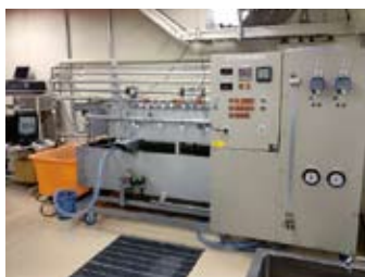
▲ 管摩擦実験装置 Pipe-friction experimental device
